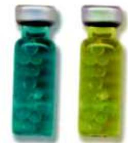
The Sonocheck is put in an empty tank. Record the time the SonoCheck changes color ( it can turn as quickly as 10 seconds). Color change should be from green to yellow. No color change you need to service the equipment. Sonocheck is easy and quick to use.
